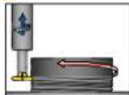
Left Hand Thread-Comb Milling
