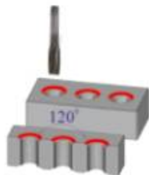
Chamfer with 120° used for tap holes, which reduce the loss of threads.
