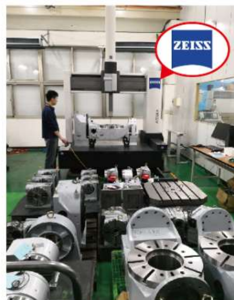
3D measuring equipment Geometry precision testing
