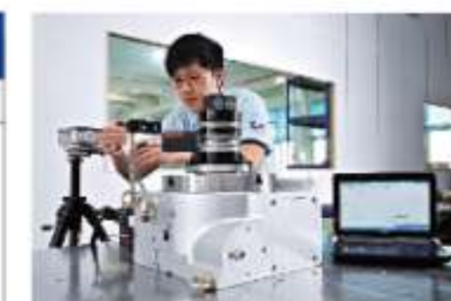
Laser measuring equipment [Indexing precision testing]
