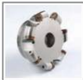
APM00-0100-0101, with 45 degree approach angle, using 16 cutting edge insert with super edge. Used in finish milling the flange face of turbocharger casing.
