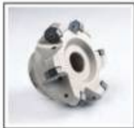
APM00-0100-0101 face milling cutter with hardfaced inserts, 16 cutting edges, with nanostructured PVD coating. Used in rough milling the flange face, with a high performance/price ratio.
