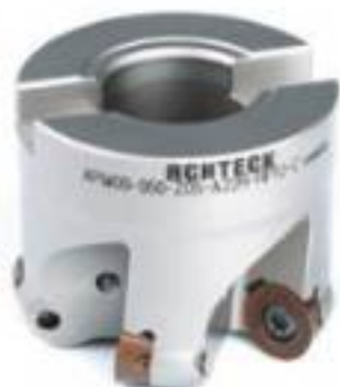
AP100-900-12 cutter used in rough milling of blade shroud.
