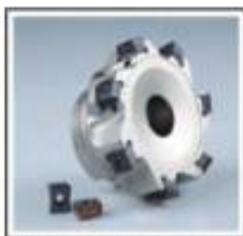
ASM90-L113 square shoulder milling cutter with tangential mounted inserts. The insert has 4 cutting edges, can be used to machine the boss surface on the turbocharger.
